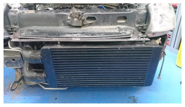
**Warning:** You can't really drive the car like this until it has been remapped, this is because the turbo settings and the map sensor, and injectors are not for this ecu setup. You can either send your ECU to us in the post, or you can program the ECU yourself using BDM100 or Kess V2. This is the better option, and then if you need to make any alterations to the software you can easily reflash it.
