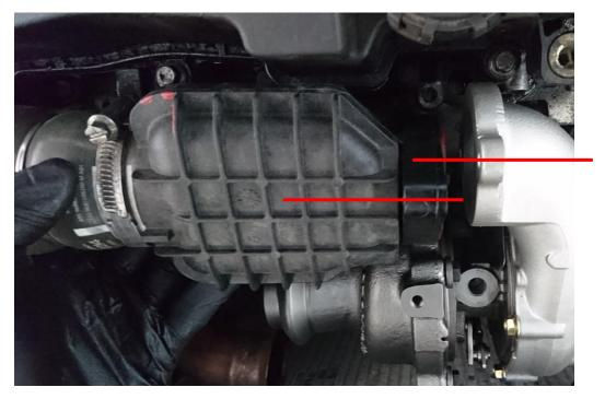
Start by removing the 10mm bolts which hold the turbine housing to the core. When these are out, carefully remove the core by puling apart. Watch for the order or the spacer shims so that you can put them back in the correct configuration, these will shoot out as they are sprung.
