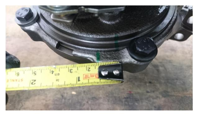
As you have now rotated the core, you also need to check that the oil drain pipe has sufficient clearance relative to the exhaust manifold. This is extremely important to avoid a fire, you do not want the drain hose to be in contact with the exhaust manifold.
