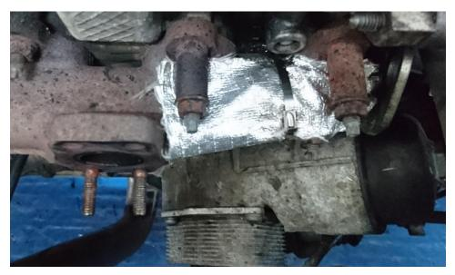
Fit the turbo using a new exhaust manifold gasket.
