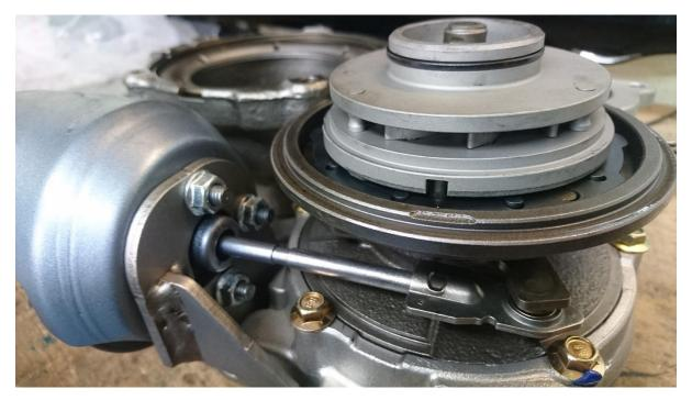
Pull out the alignment pin, this is what locks the core in to position. |You can now refit the two parts together and the will rotate freely amongst each other.
